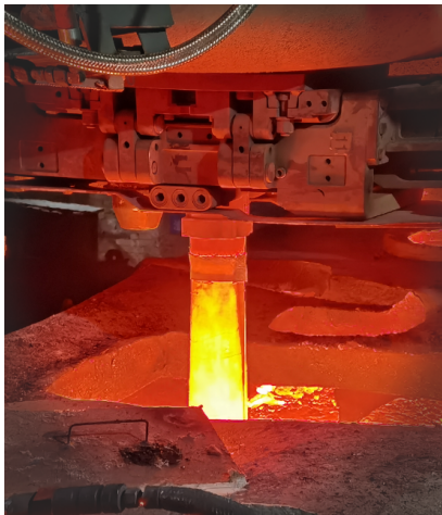
Figure 2: Ladle shroud in operation. Picture liberally taken from the Vesuvius website: www.vesuvius.com
